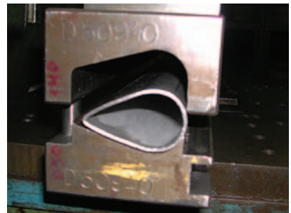
Tubes cross sections can be changed by pressing them in a die.
