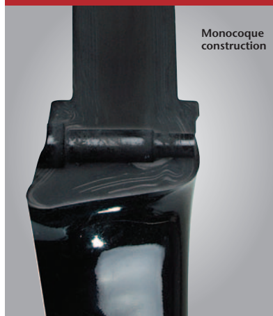
Cross-sectional views of some popular forks showing three different construction techniques.
