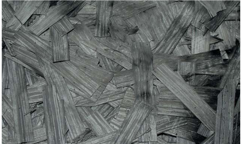
Easton Matrix Composite is comprised of extra-long, interlocking graphite fibers in a resin matrix. The prepreg sheets are laid out in a random overlapping pattern. This ensures uniform strength throughout.
