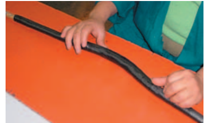
Pre-preg sheets are laid up by hand around an inflatable bladder.
