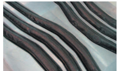
These hand lay-ups are then inserted into a mold for forming.
