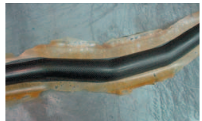
The bladders are inflated under high-pressure forming the material to the shape of the heated mold.
